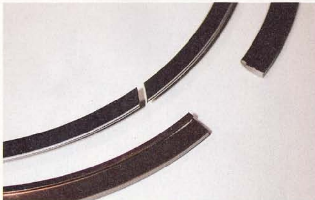
Total Seal's Gapless rings actually arrive at their Gapless status by employing a two-piece ring assembly. The main ring (foreground) is machined to accept a secondary rail segment (background) which seals the gap.
